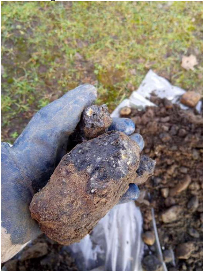
Asfalt in boring 225
