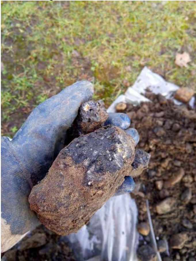
Asfalt in boring 225
